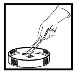
A vibrating tuning fork produces ripples in a shallow pan of water.
